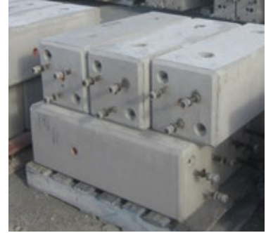
Light pole bases 67
