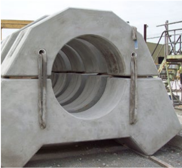
Pipeline anchor blocks
